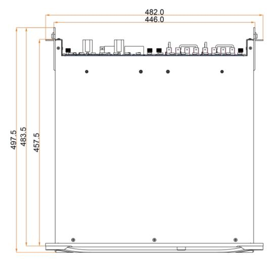
Tolerance: ±0.3 Unit: mm
